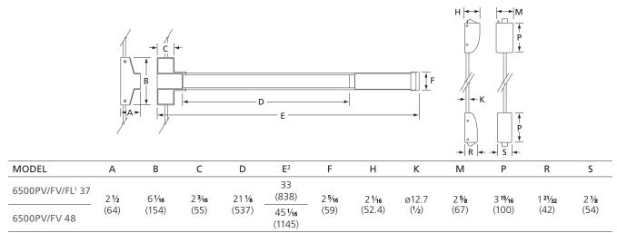
IN(MM) (1) FL MODEL DOES NOT INCLUDE BOTTOM ROD AND LATCH (2) CAN BE CUT TO SIZE - SEE PRODUCT INSTALLATION INSTRUCTIONS
